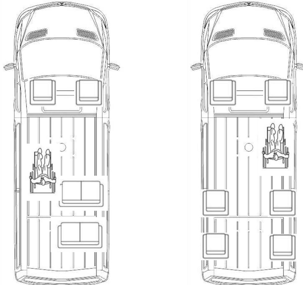
\*All standard built vehicles equipped with removable front seats to enable occupant to travel as driver or passenger, powered restraints fitted to passenger position with manual rear restraints and seatbelt stalk. Drivers and second row restraints equipped according to clients specific needs and not included in base vehicle price.
